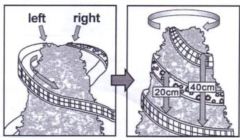
**B. Bind string lights:** Find and carefully draw out the output wire of revolving unit (9) and its wire joint ③ from the interior side of the top. Take out the LED string (12) and well connect its wire joint ④ with the wire joint ③. Then, hide the connector ③ and ④ carefully, and fix it on the interior branches, so as to avoid its entanglement with fixed objects inside the tree.
